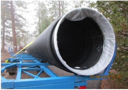
AID MCPH2 - 54-IN ID profile wall HDPE, RSC400, PE4710, ASTM F894 (1) 01-06-25
