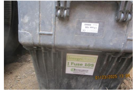
AID MCPH2 Seg2 - Sta. 846+33 54-IN ID profile wall HDPE pipe IntegriFuse Electrofusion Processor Serial 00665 (1) 01-23-25
